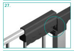
Door will be properly locked when handle hook and bottom locking bar have engaged. Test to ensure door is locked.
